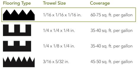
The trowel notches referenced are those typically recommended for the type of flooring being installed. They are normally the minimum size recommended. Surface conditions (roughness and porosity of substrate), type of flooring and backing will ultimately determine the required trowel notch size and coverage. Always check with the specific flooring manufacturer's recommendations for their specific trowel requirements. Ensure 100% transfer of adhesive to the substrate and the flooring backing.
